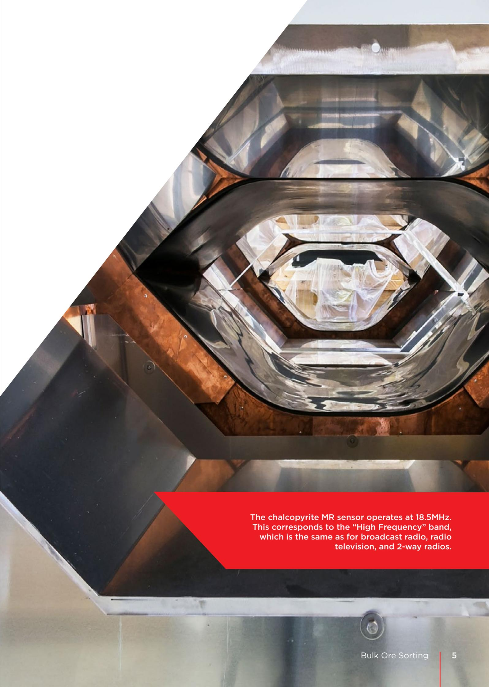
The chalcopyrite MR sensor operates at 18.5MHz. This corresponds to the “High Frequency” band, which is the same as for broadcast radio, radio television, and 2-way radios.
