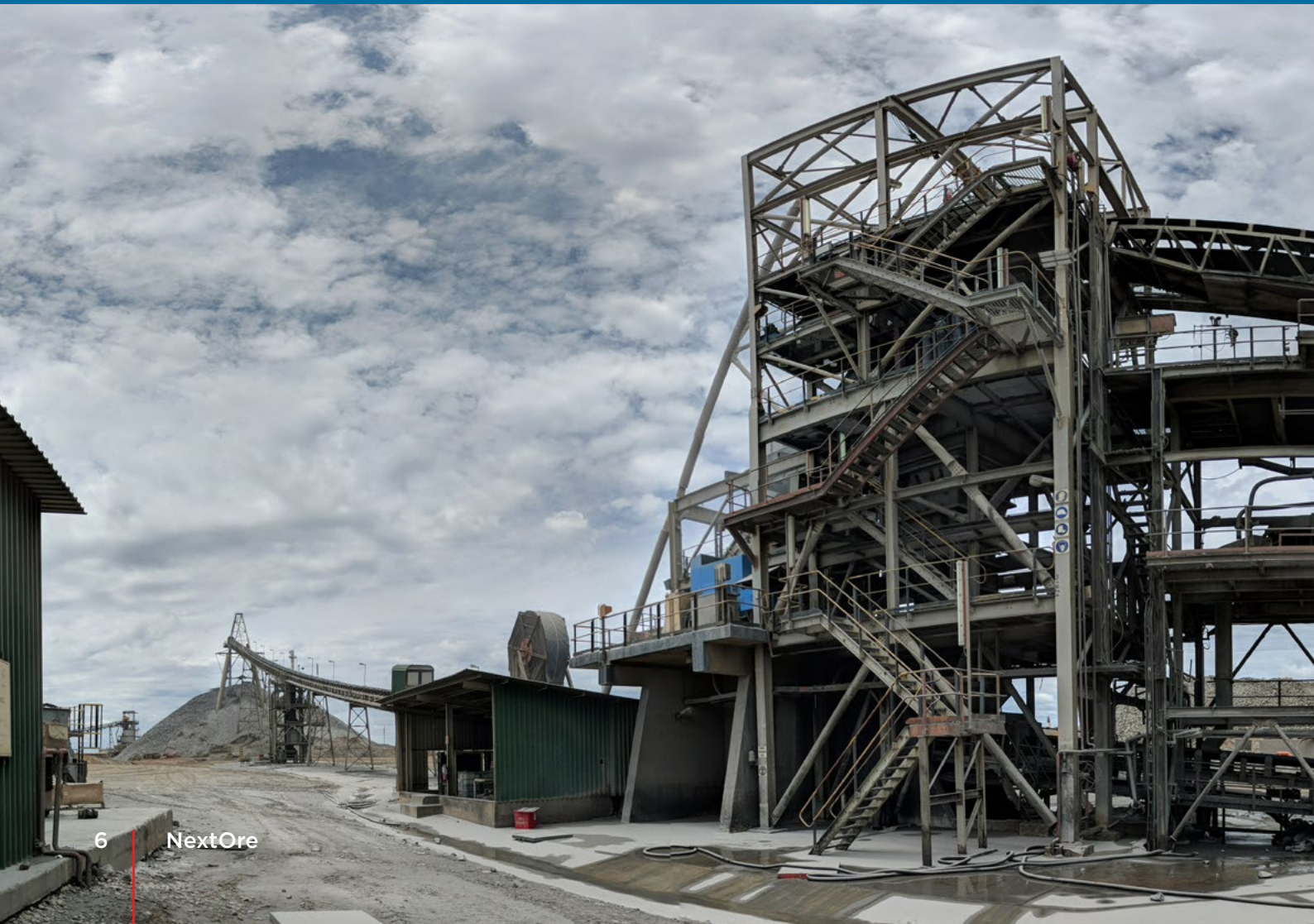
Figure 2 - Kansashi S2 primary gyratory crusher (far right), discharging to CV-1201, transfer tower and cone crusher (centre) discharging to coarse ore grinding feed stockpile (left). Photo taken prior to analyser and bulk sorting retrofit.
